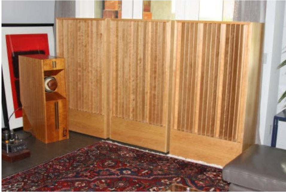
Our Quadratic Diffuser Absorber units in a customer's house. These units are an acoustic industry first marrying low frequency absorption with Quadratic Diffusion.
